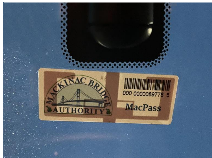
Figure 7-1. MacPass 6C Protocol Transponder
