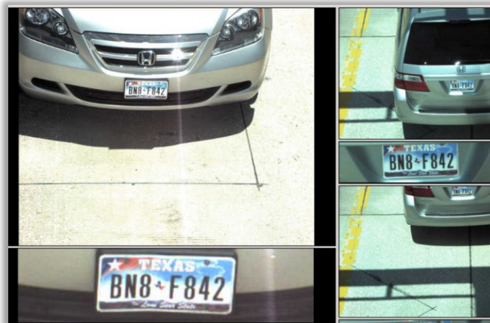
Figure 2-7: Example Images Captured by Toll Zone Electronic Toll Collection System Cameras
